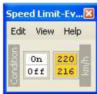
Figure 109: LIMITS – tuned SPEED LIMIT, Evo9
