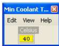
Figure 17: FUEL TUNING – tuned OPEN LOOP TEMP THRESHOLD, Evo9
