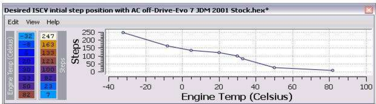
Figure 129: IDLE CONTROL – IDLE v TEMP STEPPER MOTOR TARGET AC OFF, Evo7
