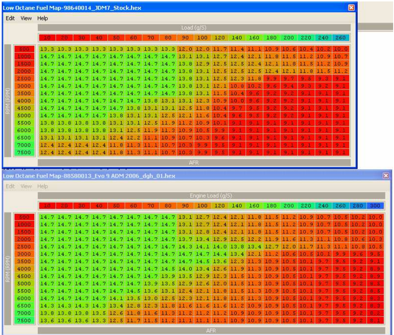
Figure 10: FUEL TUNING - LO-OCTANE FUEL MAPS, EVO7-8 and EVO9
