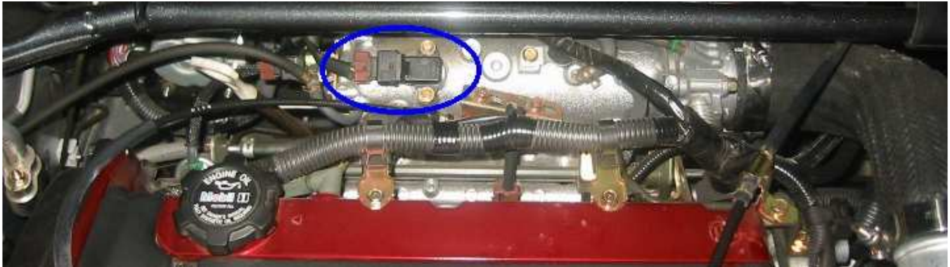
Figure 145: USDM EVO9 ENGINE & 3 BAR MAP SENSOR
