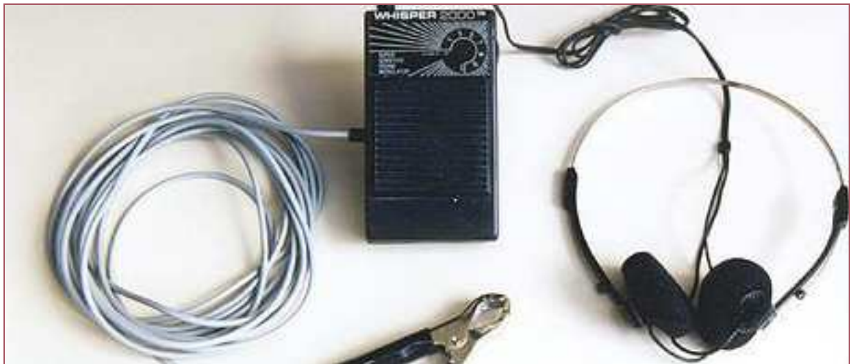
Figure 99: KNOCK TUNING, ELECTRONIC DET-CANS
