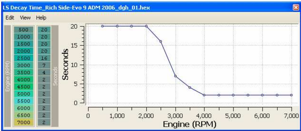
Figure 92: LEAN SPOOL - TRANSITION TIME RICH SIDE v RPM, Evo9
