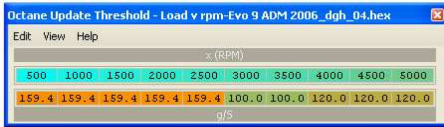
Figure 97: KNOCK TUNING – OCTANE UPDATE THRESHOLD, Evo9
